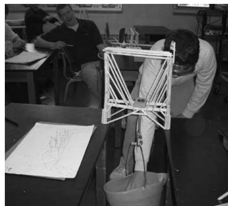
Eric Abrahamian '10 added weight to the bucket to test the efficiency ratio of the bridge.
